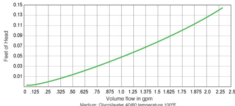
Feet of head curve for 1 foot of 3/4" SolarFlex
